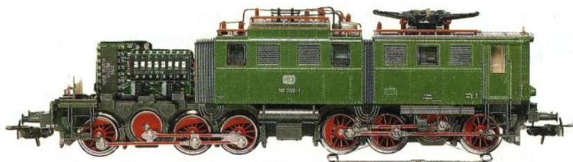
Locomotive with c 80 decoder installed
